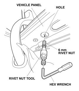
6. While holding the rivet nut tool with the hex wrench, turn the 19 mm wrench counterclockwise to install the 6 mm rivet nut to the vehicle panel.
