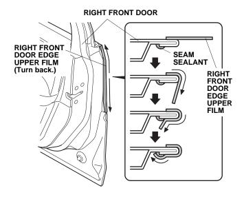
8. Wipe up the water on the right front door edge upper film using a shop towel. Allow the right front door edge upper film to dry thoroughly.
