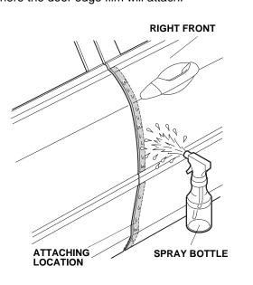
3. Open the right front door again. Peel back about 50 mm (2 in.) of adhesive backing from the right front door edge upper film. Align the V-notch in the right front door edge upper film with the end of the character line on the upper part of the right front door.
