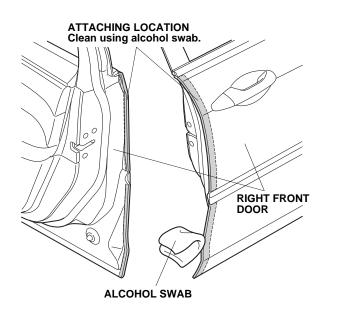
Close the right front door. Using a spray bottle with 3M protective tape application solution, spray the area where the right front door edge film will attach. NOTE: Do not spray the inner surface of the door where the door edge film will attach.
