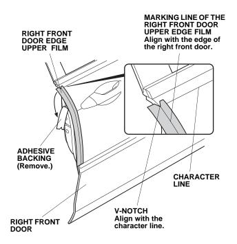
4. Continue to remove the adhesive backing while you align the center line on the door edge film with the edge of the door.
