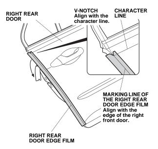
On the right rear door, you will have to lift the door seal to fold the right rear door edge film onto the inside of the right rear door. Take care not to damage the door seal.
