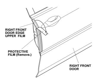
7. Starting from the middle and working outward, fold over back the right front door edge upper film onto the inside of the right front door as shown. Move your fingers in one direction only. Take care not to damage the door seal.
