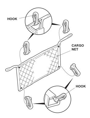
12. Install the cargo net to the tie down hooks and the anchors in the trunk. The cargo net can be installed in two different positions, vertically or horizontally.
