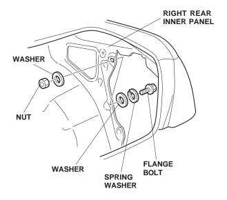
8. Reinstall all removed parts. Check that all clips are installed securely.
