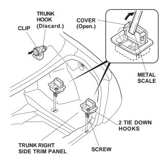
4. Remove the trunk hook (clip) from the trunk right side trim panel.
