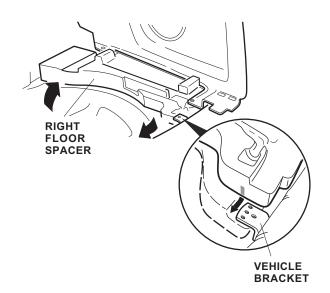
32. Loosely install one 6 x 20 mm flange bolt into the right jack nut.
