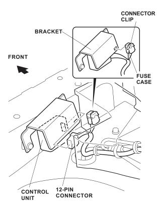
35. Rotate the control unit assembly down onto the right flange bolt. Torque both  $6 \times 20$  mm flange bolts to 4.0 N·m (3.0 lb-ft).
