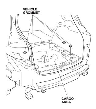
38. Insert the right and left plates into the holes exposed in step 40.
