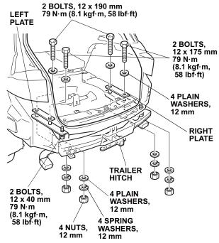
41. Torque the 12 x 40 mm bolts installed in step 39 to 79 N·m (58 lb-ft).
