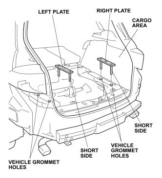
39. Install the trailer hitch with two 12 x 40 mm bolts with plain washers and lock washers but do not tighten the bolts yet.
