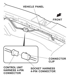
25. Secure the socket harness 4-pin connectors to the vehicle panel using the connector clip.
