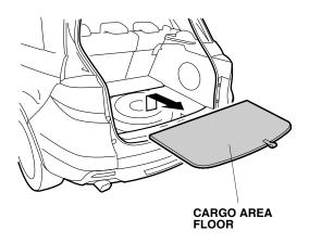
5. Remove the cargo area floor board (four clips).
