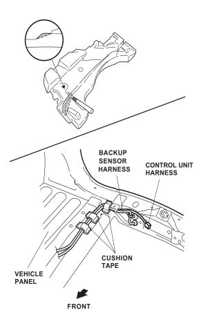
24. Plug the control unit harness 4-pin connector into the socket harness 4-pin connector.
