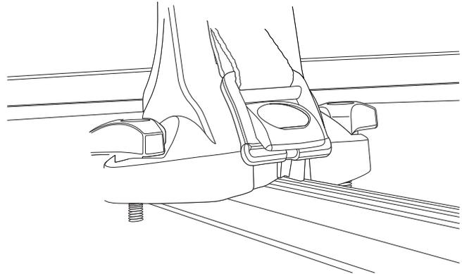
8. Pull the end of the attachment straps to secure the surfboard to the carrier. Make certain all mounting hardware is secure, then tighten as necessary.
