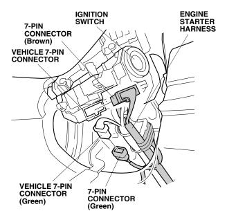
32. Plug the engine starter harness 7-pin connector (brown) into the vehicle 7-pin connector.
