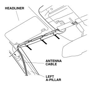
64. At the left A-pillar, route the antenna cable down along the vehicle harness. Align the mark you made on the antenna cable with the lower vehicle clip, and secure the antenna cable to the vehicle harness with one wire tie.
