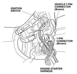
29. Plug the engine starter harness 7-pin connector (green) into the vehicle 7-pin connector.
