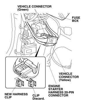
44. Route the engine starter harness 20-pin connector to the position under the fuse box.
