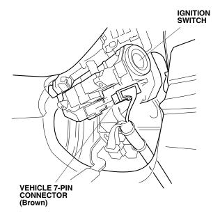
27. Route the engine starter harness to the ignition switch.
