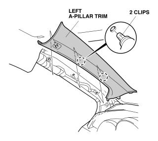
13. Remove and discard the pillar clip from the left A-pillar, and install a new pillar clip (supplied) on the left A-pillar trim.
