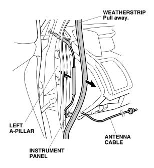
67. Under the instrument panel, secure the antenna cable to the vehicle harness with two wire ties.
