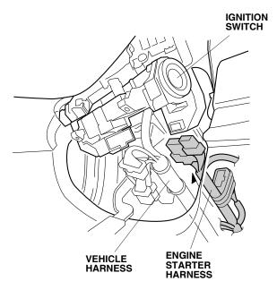
28. Plug the vehicle 7-pin connector (brown) into the engine starter harness 7-pin connector (brown) and route the engine starter harness as shown.
