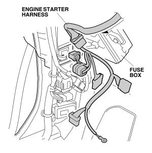
41. Unplug the vehicle 18-pin connector (white) located inside the vehicle frame, and plug the engine starter harness 18-pin connector into the vehicle 18-pin connector. Plug the vehicle 18-pin connector you just unplugged into the engine starter harness 18-pin connector.
