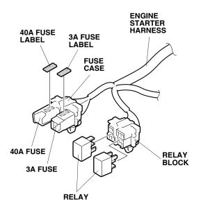
24. Attach the 3A fuse label and the 40A fuse label to the engine starter harness fuse case.
