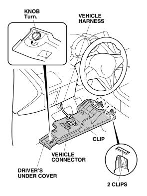
18. Release the vehicle harness (one clip) and remove the driver's under cover (unplug the vehicle connector).
