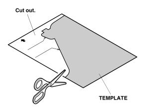
52. Using isopropyl alcohol on a shop towel, clean the windshield surface where the template will attach. Position the template on the black painted surface of the front windshield by aligning its edges with the contour of the black painted area. Secure the template to the windshield using masking tape.
