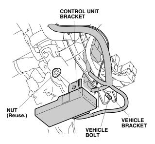
73. Starting at the control unit and working toward the fuse box, secure the engine starter harness and the antenna cable to the vehicle harness at the green tape with one wire tie.
