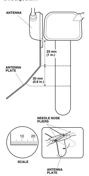
57. Attach one piece of urethane tape (cut in step 54) to the antenna plate as shown. Trim to fit.
