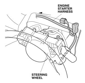
34. Unplug the vehicle 12-pin headlight switch connector. Plug the engine starter harness 12-pin connector into the headlight switch connector. Plug the vehicle 12-pin headlight switch connector you just unplugged into the engine starter harness 12-pin connector.
