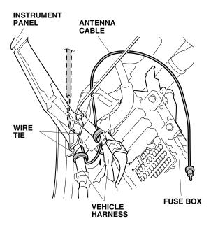
68. Continue routing the antenna cable to the engine starter harness relay block along the engine starter harness.
