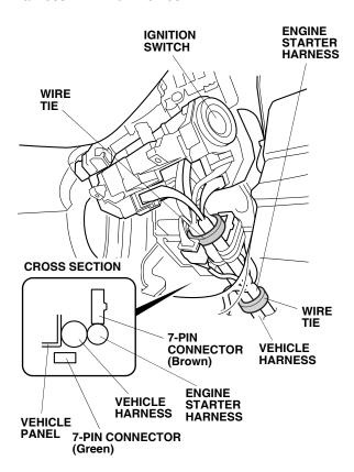
39. Attach the engine starter harness relay block and engine starter harness fuse case to the vehicle bracket.
