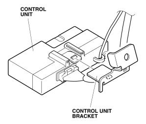
72. Remove the nut from the vehicle bracket, and install the control unit bracket onto the vehicle bracket.
