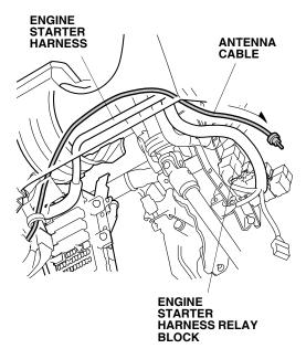
69. Plug the antenna cable terminal into the control unit.
