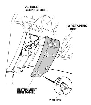
17. Release the driver's under cover (turn the knob counterclockwise, and disconnect two clips).
