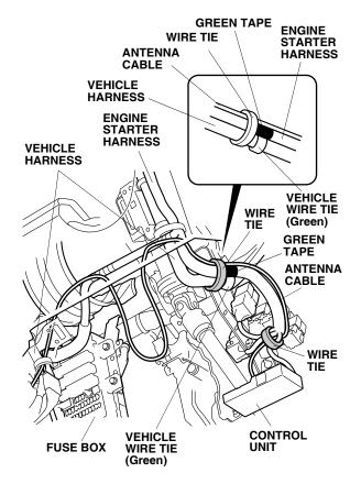
74. Continue routing the antenna cable toward the fuse box, and secure the antenna cable to the vehicle harness with one wire tie near the fuse box. Allow the excess harness to hang between the two wire ties.
