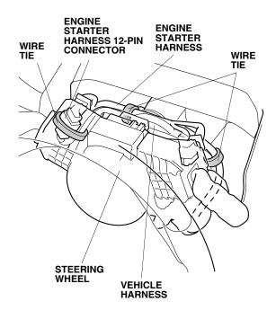
37. Secure the engine starter harness to the vehicle harness with two wire ties.
