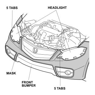
13. Pull the mask back toward the left fenderwell, smooth out any wrinkles, and snap the mask onto the snap-screw.
