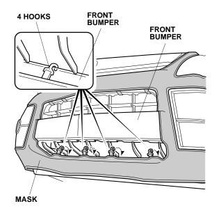
19. Attach the five bottom hooks to the bottom edge of the front bumper.
