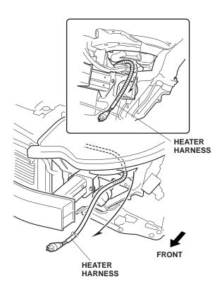
18. Secure the fifth wire tie with clip to the vehicle frame.
