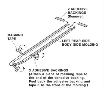
10. Align the front edge of the left rear side molding with the rear template as shown, and temporarily attach it using the top edge of the template as a guide.
