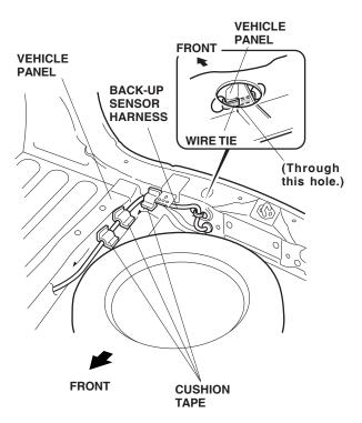
28. Route the back-up sensor harness forward and secure it to the vehicle panel with two cushion tapes.
