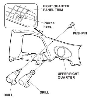
42. While wearing eye protection, drill a 19 mm hole in the outside surface of the right quarter panel trim at the pierced point. Remove all burrs.
