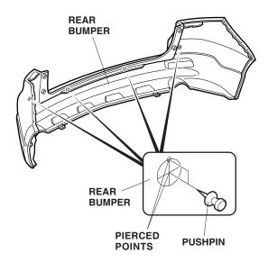
22. While wearing eye protection, drill a 3 mm pilot hole through the outside surface of the rear bumper at each of the eight pierced points you just made.
