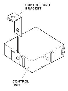
40. Plug the back-up sensor harness 14-pin connector into the control unit and install the control unit bracket to the vehicle panel with the special screw.
