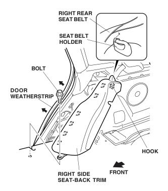
11. Remove the right side seat-back trim (one bolt and one hook) and remove the right rear seat belt from the seat belt holder.
