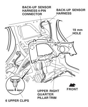
44. Plug the back-up sensor harness 4-pin connector into the switch, and install the switch into the 19 mm hole in the direction shown.
