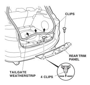
7. Remove the two clips from the rear trim panel. Remove the rear trim panel (four clips).
