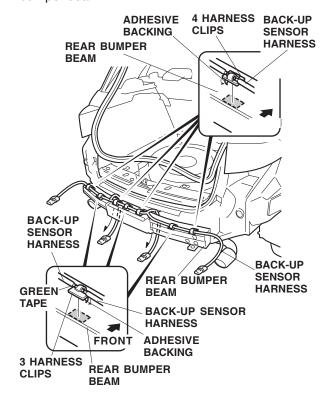
47. Attach the seven harness clips to the back-up sensor harness. Three of the clips attach at the green-taped locations. Using isopropyl alcohol on a shop towel, clean the rear bumper beam where the harness clips attach. Remove the adhesive backings from the seven harness clips, and attach them to the rear bumper beam in the area shown. Start at the center and work your way outward on each side.
