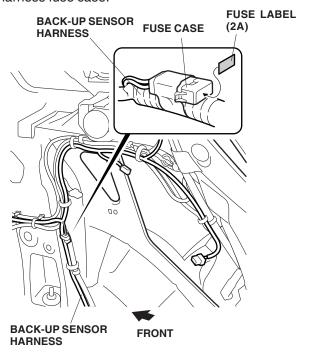
38. Plug the back-up sensor harness 2-pin connector into the vehicle 2-pin connector.
