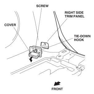
14. Remove the bolt cover from the right side trim panel, and remove the two bolts and three clips.
