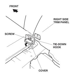
13. Open the right rear tie-down hook cover. Remove the rear tie-down hook from the right side trim panel (one screw).
