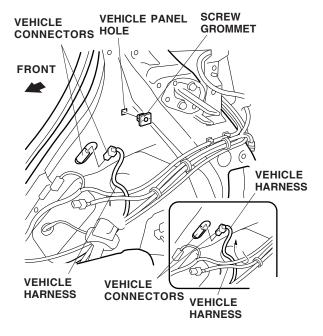
32. Disconnect the vehicle connector. Inside the vehicle panel, route the vehicle harness under the existing vehicle connector running along the fenderwell panel and reconnect the vehicle connector. 33. Using isopropyl alcohol, thoroughly clean the vehicle panel area where the cushion tape will attach. Secure the back-up sensor harness to the vehicle panel with one cushion tape.
