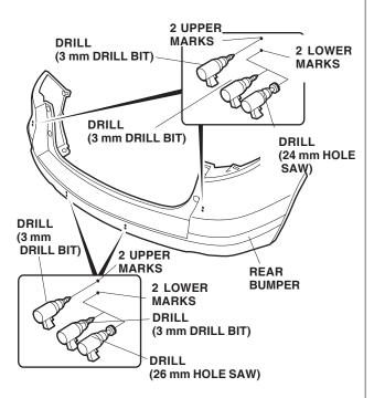
23. While wearing eye protection, enlarge the lower hole at each of the marks using a 24 mm hole saw (outer holes) and a 26 mm hole saw (inner holes). Remove all burrs.
