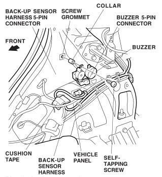
34. Plug the back-up sensor harness 5-pin connector into the buzzer 5-pin connector and secure the buzzer to the screw grommet with the self-tapping screw and collar.
