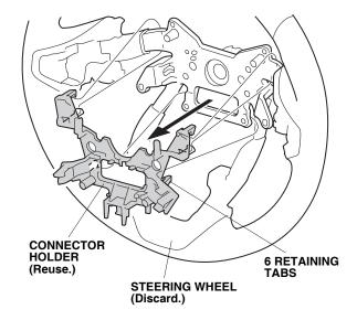
16. Install the connector holder on the new steering wheel.
