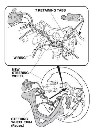
18. Secure the ground wire with the screw, and attach the wiring to the retaining tab.
