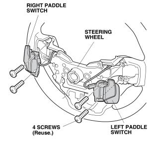
12. Remove the two self-tapping screws from the steering wheel.
