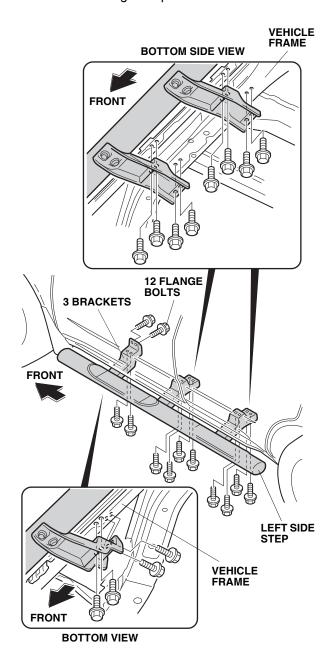
2. Torque the six flange bolts already attached to the left side step to 27 N·m (20 lbf·ft).
