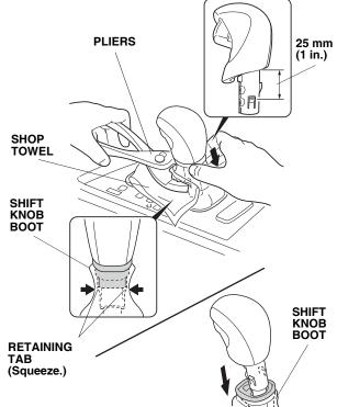
3. Remove the two screws from the shift knob, and remove the shift knob by pulling it up.
