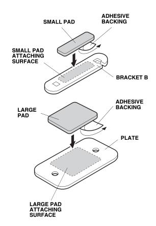
5. Using isopropyl alcohol on a shop towel, clean the four plates where the large pads will attach. Remover the adhesive backings from the large pads and attach them to the plates.
