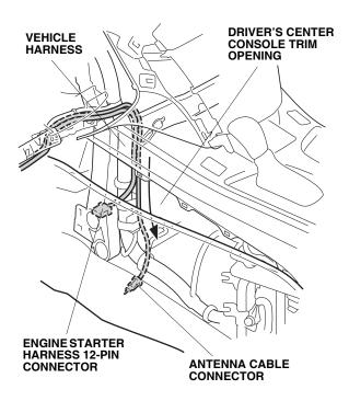
61. Secure the engine starter harness and antenna cable to the dashboard frame with three wire ties.
