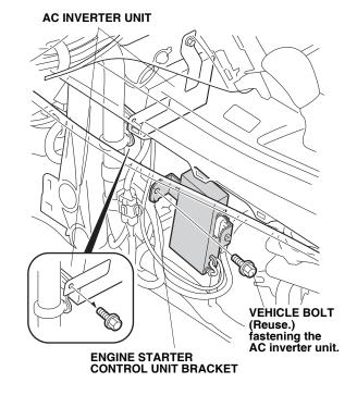
77. Install the clip on the engine starter subharness 12-pin connector to the engine starter control unit bracket as shown.
