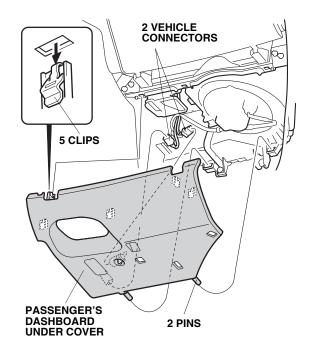
20. Remove the right front door sill trim (four clips, two retaining tabs and two pins).
