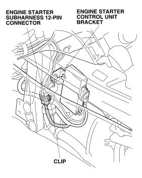
78. Secure the engine starter harness, engine starter subharness, and antenna cable to the vehicle harness with two wire ties as shown. Bundle the excess antenna cable and secure it using one wire tie as shown.
