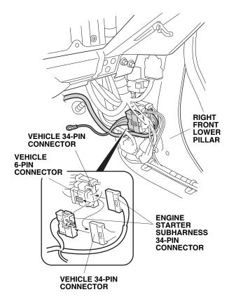
64. Unplug the vehicle 34-pin connector, and plug the engine starter subharness 34-pin connectors in between.
