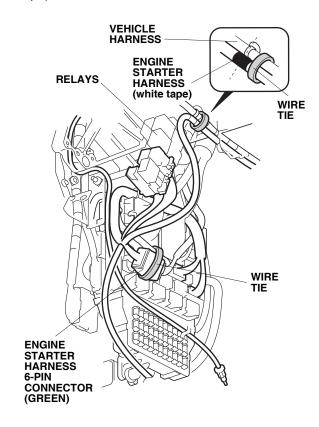
58. Secure the engine starter harness and antenna cable to the vehicle harness with one wire tie.
