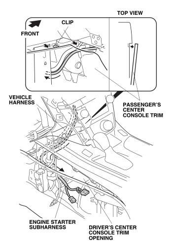
70. Secure the engine starter subharness to the vehicle harness with four wire ties in the areas shown.
