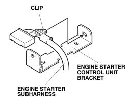
73. Install the engine starter control unit bracket and plug the engine starter subharness 28-pin connector into the control unit. Note the direction of the bracket.
