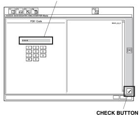
11. Check that "The registration of the Remote Control Engine Starter Unit has been completed" is shown, then click the check button.
