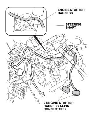
49. Directly behind the steering shaft, unplug the vehicle 22-pin connector and 6-pin connector for access, and the vehicle 14-pin connector (white).
