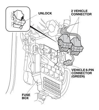
41. Unplug the vehicle 6-pin connector (green) from the fuse box.
