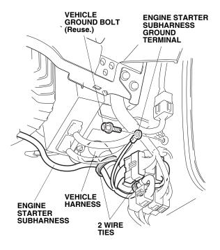
67. Secure the engine starter subharness to the vehicle harness with two wire ties.
