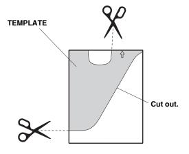
26. Secure the template to the windshield with the masking tape while aligning it with the edge of the black ceramic part as shown.
