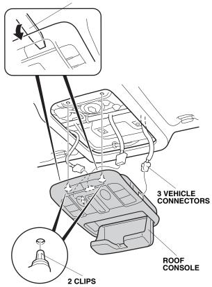
7. Remove the sunvisor holders. Using a flat-tip screwdriver, push the hook, and turn the holder 90°, then pull it out.
