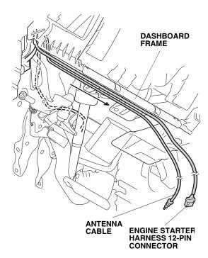
60. At the center console, route the engine starter harness 12-pin connector and antenna cable connector down along the vehicle harness to the driver's center console trim opening.
