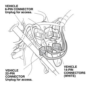
50. Plug the engine starter harness 14-pin connector into the vehicle 14-pin connector and plug the vehicle 14-pin connector into the engine starter harness 14-pin connector.
