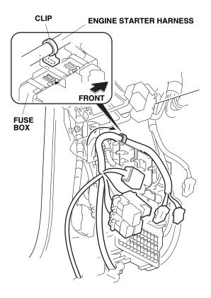
43. Plug the engine starter harness 6-pin connector (green) into the fuse box, and plug the vehicle 6-pin connector (green) into the engine starter harness 6-pin connector (green).
