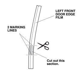
6. Partially peel back the adhesive backing from the upper part of left front door edge film. Align the V-notch in the upper part of door edge film with the end of the character line on the driver's door.
