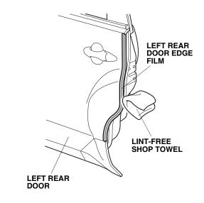
22. Repeat steps 14 thru 21 to install the right rear door edge film on the right rear door.
