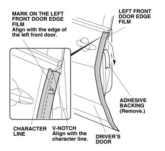
4. Continue to remove the adhesive backing while you align the mark on the left front door edge film with the edge of the driver's door. Go to step 9.
