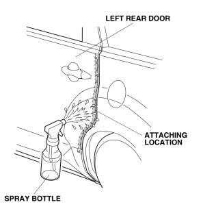
16. Open the left rear door again. Peel back about 50 mm (2 in.) of adhesive backing from the left rear door edge film. Align the V-notch in the door edge film with the end of the character line on the upper part of the left rear door.
