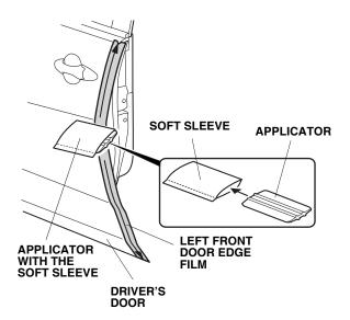
10. When you are satisfied that the door edge film is firmly attached to the edge of the driver's door, slowly remove the outer protective film.
