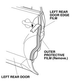
20. Starting in the middle of the door edge film and working outward, fold the door edge film around the edge of the left rear door using your fingers. Move your fingers in one direction. Attach the door edge film over the seam sealant. Do not trim or damage the seam sealant.
