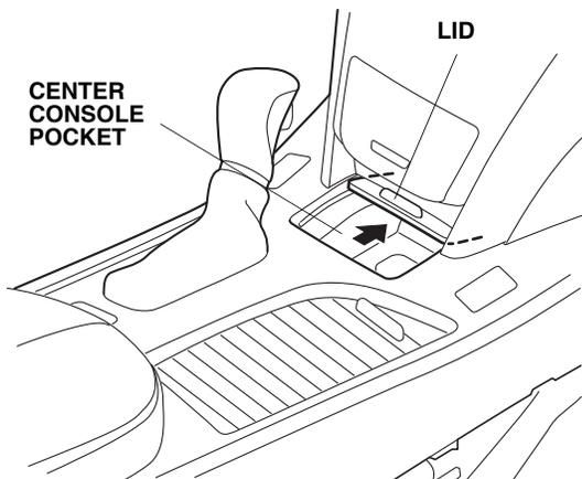
6. Open the accessory socket lid. Remove the accessory socket by reaching in from the driver's console trim opening and pushing up on the accessory socket. Use a 90° awl to release the two retaining tabs.
