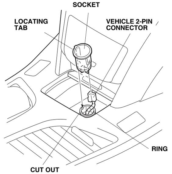
11. Align the locating tab on the socket with the cutout in the ring, and slide the socket into the ring.
