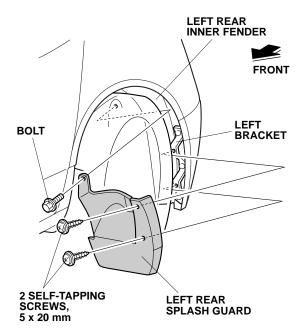
5. Secure the left rear splash guard to the rear bumper with one clip.
