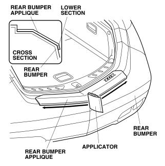
10. Slowly remove the protective film from the rear bumper applique. Remove the film horizontally, do not pull up.
