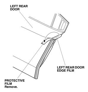
28. Starting from the center and working outward, use the applicator and sleeve to fold the left rear door edge film inside the left rear door as shown. Move the sleeve in one direction only. Do not damage the door seam sealant. Pull back the molding on the left rear door.
