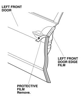
17. Starting from the center and working outward, use the applicator and soft sleeve to fold the left front door edge film inside the left front door as shown. Move the applicator in one direction only. Do not damage the door seam sealant. Pull back the molding on the left front door.
