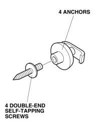
5. Install two anchors into the left and two anchors into the right rear side trim panels.
