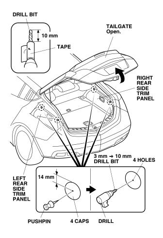
3. While wearing eye protection, drill two holes in the left and two holes in the right rear side trim panels. To prevent damage to the inner panels, wrap tape around the end of each drill bit 10 mm away from the tip. First drill with a 3 mm drill bit, then enlarge the holes to 10 mm using a 10 mm drill bit.
