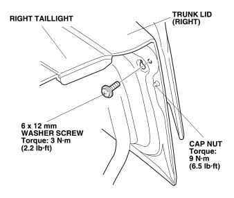
19. Torque the washer-screw to 3 N·m (2.2 lb-ft) then torque the cap nuts to 9 N·m (6.5 lb-ft). Reinstall the rubber stoppers you removed in step 9.
