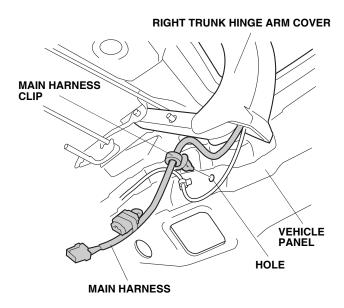
31. Unplug the vehicle 4- pin connector from the right taillight, and plug the main harness 4-pin into the taillight. Plug the taillight 4-pin connector into the main harness 4-pin connector.
