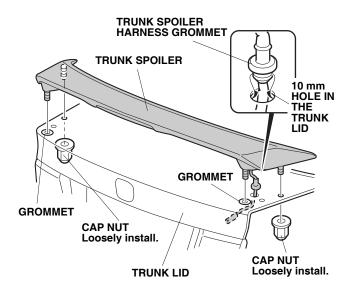
18. On each side install one 6 x 12 mm washer screw into the trunk spoiler.
