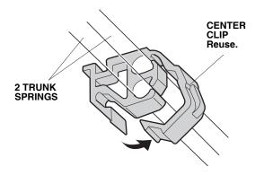
37. With an assistant holding the trunk lid open, remove the old trunk springs from the trunk hinge arms using the trunk spring tool. Wear gloves to protect your hands, and pull the trunk spring tool slowly and carefully towards you.)
