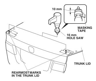
16. Install one grommet into each 16 mm hole in the trunk lid.
