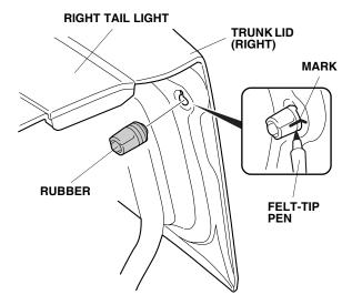
On the inside of the trunk lid, locate the two identification marks on the trunk lid. Lightly centerpunched each mark. Repeat on the left side of the trunk lid.
