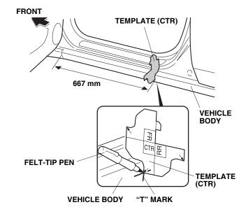
3. Open the left rear door. Position the template (marked RR) on the vehicle body. Using a felt-tip pen, mark the vehicle body at the measurement shown.
