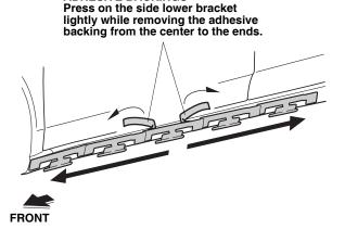
13. While wearing gloves, adhere the side lower bracket by firmly pressing on the double-sided tape. Take care not to press on the bracket mounting plates as it can deform the plates. The side under spoiler cannot be installed securely if the mounting plates are bent.
