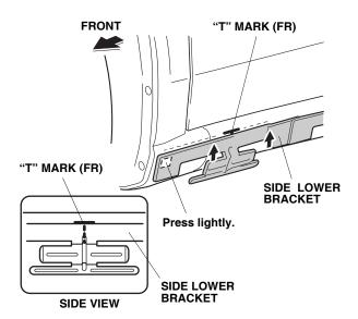
Raise the rear of the side lower bracket to contact the "T" mark (RR). Press on the rear of the bracket (where you removed the adhesive backing) firmly to adhere.
