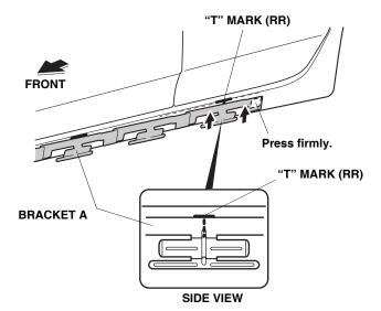
10. Temporarily detach the front end of side lower bracket where you lightly pressed in step 8. Keep holding the end of the bracket. Position the top of the bracket to the "T" mark (FR), and press on the front of the bracket firmly to adhere.
