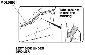
17. Pull the left side under spoiler lightly toward you and check that all the five resin brackets fit on the side lower bracket mounting plates securely. Visually check that the left side under spoiler is installed securely. If it is loose, repeat the installation procedure.
