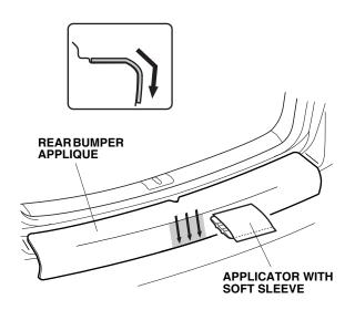
11. Use the applicator with soft sleeve to apply the rear bumper applique to the rounded rear edge on the left side as shown. Start in the middle and work outward. Repeat for the right side.
