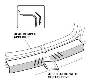
12. Remove the protective film from the top rear bumper applique. Slowly pull the protective film back. Avoid pulling it upward.
