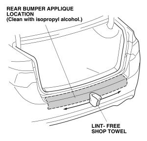
3. Using a spray bottle with protective tape application solution, spray the rear bumper where the rear bumper applique will attach.
