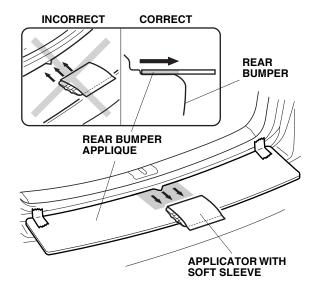
8. Starting from the center and working outward, use the applicator with soft sleeve to smooth the rear bumper applique. Repeat on the right side. Stroke in one direction only.
