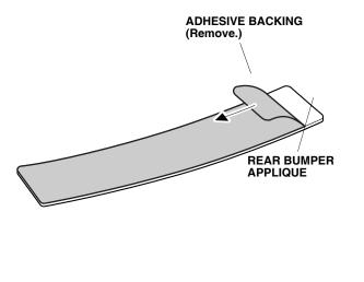
Generously apply the protective tape application solution to the adhesive side of the rear bumper applique.
