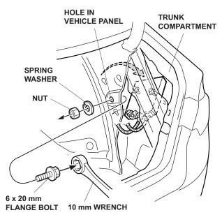
Locate the hole in the vehicle panel. Install one 6 x 20 mm flange bolt through the vehicle panel hole, then install a spring washer. Reinstall the stereo amplifier and a nut, and tighten. Be careful not to drop the bolt. 10. In the rear metal shelf, locate the hole near the trunk hinge arm.
