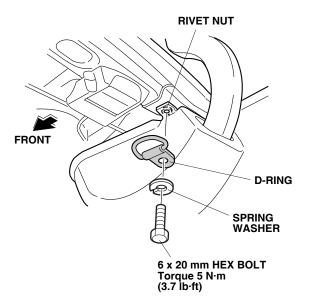
15. Remove the left trunk side trim panel, and repeat steps 5 through 13 to install a T-anchor and a D-ring on the left side of the vehicle.
