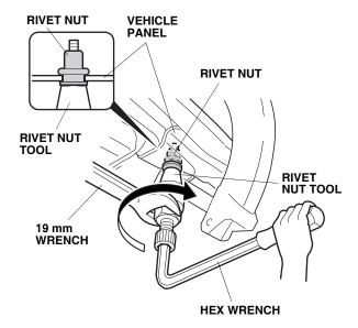
• Remove the tool from the rivet nut by turning the hex wrench clockwise.
