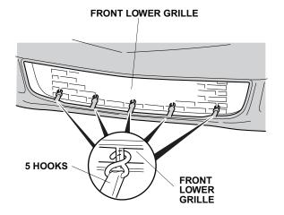
13. Secure the two hooks at the indicated locations to the front bumper. Repeat on the other side.
