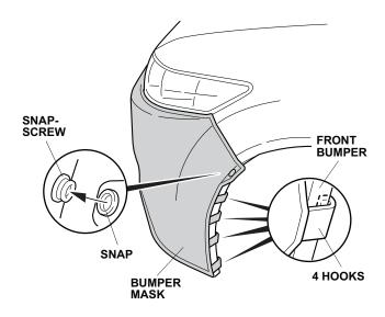
9. Insert the six tabs between the front bumper and the headlight and secure the hook at the indicated position. Repeat on the other side.
