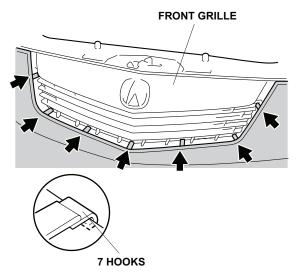
11. Secure the four hooks at the indicated locations to the front lower grille.
