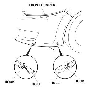
14. Secure the six hooks at the indicated locations to the front bumper.
