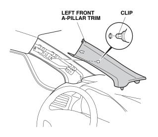
23. Remove and discard the clip from the left front A-pillar trim, and install a new A-pillar clip (supplied) on the left front A-pillar trim.
