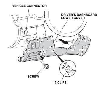
9. Remove the driver's dashboard under cover (two clips and one pin, and unplug the vehicle connector).
