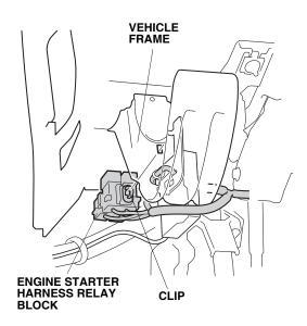
66. Bundle up the excess antenna cable, and insert the bundled cable under two wire ties loosely attached in step 59.
