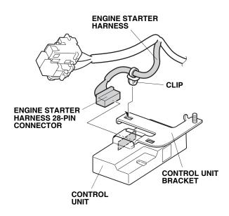
62. Install the clip from the engine starter harness to the control unit bracket.
