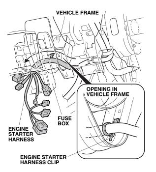
34. Attach the engine starter harness clip to the clip on the vehicle frame as shown.
