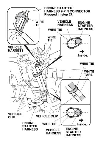
32. Align the white tape on the engine starter harness with the holes in the dashboard behind the tilt lever as shown, and secure the engine starter harness to the dashboard with one wire tie.
