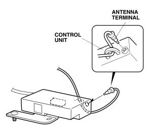
64. Insert the stud from the control unit bracket thru the hole in the vehicle frame and secure the control unit to the vehicle frame using the flange nut.
