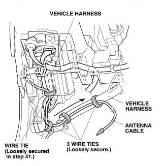
59. Route the antenna cable along the vehicle harness, and loosely secure the antenna cable to the vehicle harness with three wire ties.
