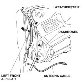
57. Secure the antenna cable to the vehicle harness with four wire ties.
