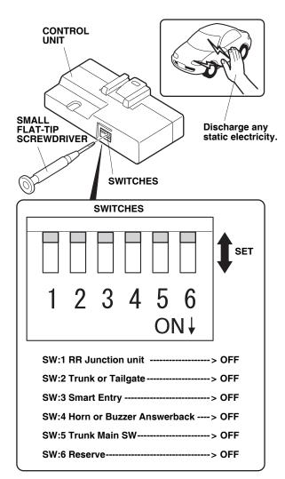
5. Check a location of the switches on the control unit. NOTE:
