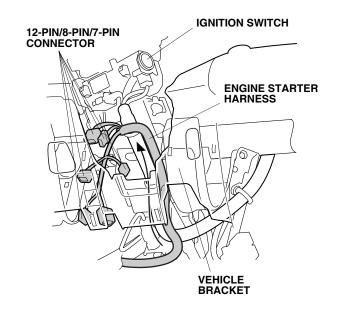
27. Unplug the vehicle 7-pin connector, and plug it into the engine starter harness 7-pin connector. Plug the remaining engine starter harness 7-pin connector into the vehicle 7-pin connector.
