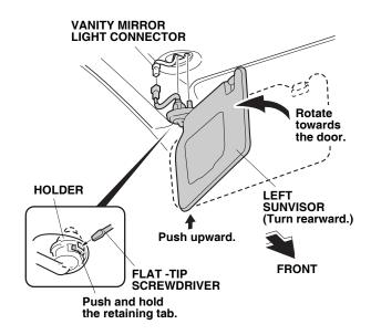
19. While holding the retaining tab, rotate towards the door to remove the left sunvisor. Unplug the vanity mirror light connector.
