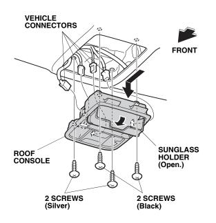
17. Turn the sunvisor holder 90°, and remove the two sunvisor holders.
