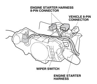
30. Secure the engine starter harness to the vehicle harness using two wire ties. Do not secure it to the SRS harness.
