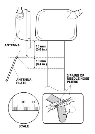
47. Get the antenna. Starting near the antenna end of the cable, wrap three urethane tapes around the antenna cable at the measurements shown.
