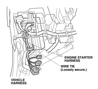
42. Unplug the vehicle 24-pin connector from the fuse box, and plug the engine starter harness 24-pin connector into the fuse box. Plug the remaining engine starter harness 24-pin connector into the vehicle 24-pin connector.
