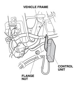
65. Clip the engine starter harness relay block to the vehicle frame.
