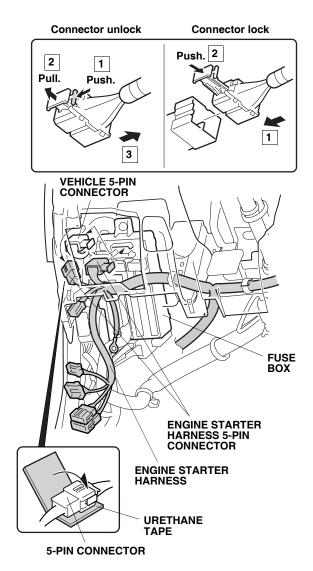
36. Plug the vehicle 5-pin connector into the engine starter harness 5-pin connector.
