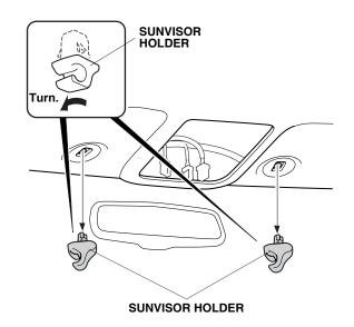
18. Locate the slot in the holder, and insert a flat-tip screwdriver into the slot. Push in and hold the retaining tab.
