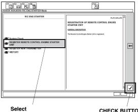
Select "REGISTER REMOTE CONTROL ENGINE STARTER UNIT." 9. Check that "Obtain PCM-code (IMMOBILIZER PCM CODE) from iN. This vehicle's VIN will be required to obtain the password. (USA)" is shown, then click the check button.
