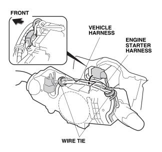
31. Align the white tape on the engine starter harness with vehicle clip as shown, and secure the engine starter harness to the vehicle harness with three wire ties in the areas shown.
