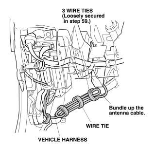
67. Secure the antenna cable to the vehicle harness with one additional wire tie.
