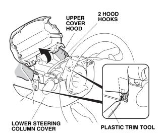
Remove the upper steering column cover from the upper cover hood (two clips)
