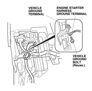
41. Loosely secure the engine starter harness to the vehicle harness with one wire tie.
