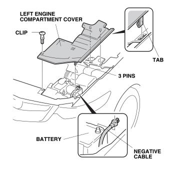
3. Disconnect the negative cable from the battery.
