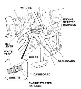
33. Route the engine starter harness through the opening in the vehicle frame in front of the fuse box.
