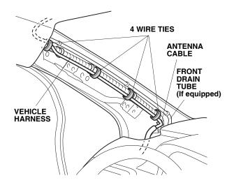
58. Secure the antenna cable with the one wire tie loosely secured to the vehicle harness in step 41.
