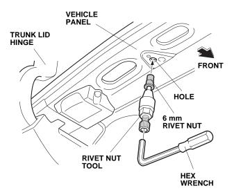
3. Hold the rivet nut tool with the hex wrench, and turn the 19 mm wrench counterclockwise to install the 6 mm rivet nut into the vehicle panel.
