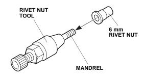
2. Open the trunk lid. Insert the 6 mm rivet nut into the hole in the vehicle panel, and attach the hex wrench to the rivet nut tool.
