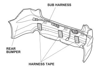
54. With the help of an assistant, bring the rear bumper close to the vehicle. Plug the sub harness 8-pin connector into the sensor harness 8-pin connector, and install the rear bumper in the original position.
