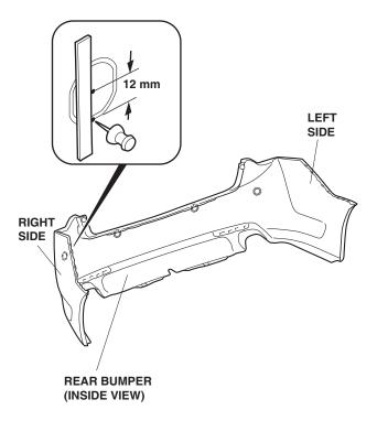
For the two center marks on the bumper, use a straight edge to measure 13 mm upward, and pierce the bumper.
