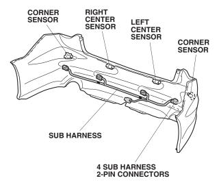
51. Align the green tape on the sub harness with the holes on the left center sensor clip and the right center sensor clip, and secure the sub harness to the left center sensor clip and right center sensor clip using two wire ties as shown.
