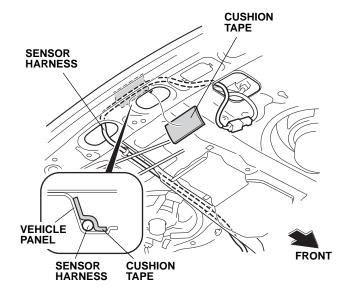
24. Secure the sensor harness to the vehicle panel using one cushion tape.
