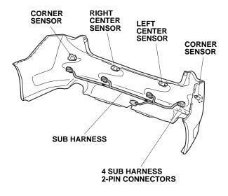
42. Align the green tape on the sub harness with the holes of the left center sensor clip and the right center sensor clip, and secure the sub harness to the left center sensor clip and the right center sensor clip using two wire ties as shown.
