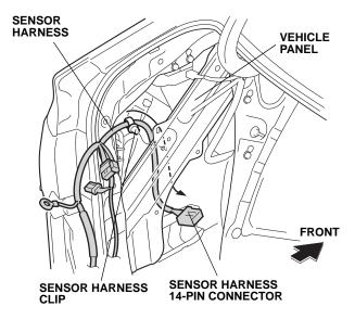
11. Secure the sensor harness clip to the vehicle panel.
