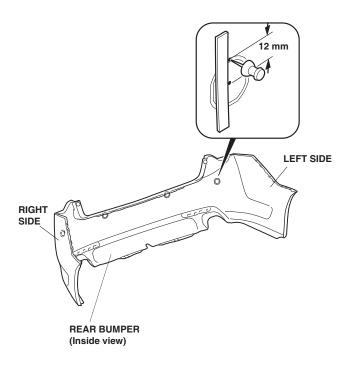
On the right side of the bumper, use a straight edge to measure 12 mm downward from the center mark, and pierce the bumper.
