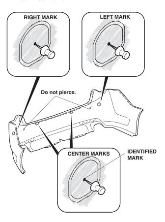
On the left side of the bumper, use a straight edge to measure 12 mm upward from the center mark, and pierce the bumper.
