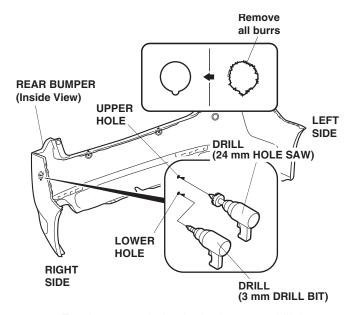
For the center holes in the bumper, drill the upper holes using a 3 mm drill bit, and drill the lower hole using a 26 mm hole saw.
