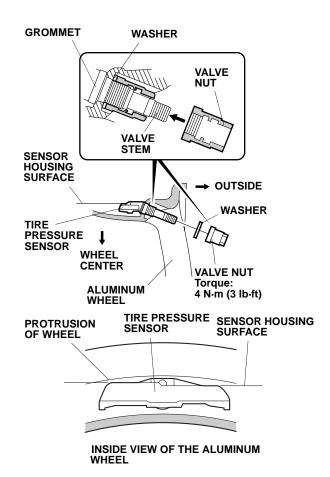
7. While holding the tire pressure sensor to keep it from rotating, torque the valve nut to 4 N·m (3 lb-ft). You may hear a snap or pop as you torque the nut; this is normal.
