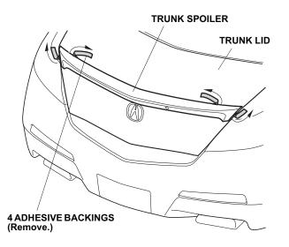
21. Using a hard rubber roller, apply pressure and roll it from one end to the other.
