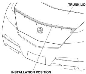
INSTALLATION POSITION (Clean with the alcohol pads.) 11. Install a thick seal, (3 mm), to each of the three grommets.
