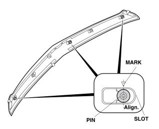
16. Center the spoiler on the trunk lid, and check the distance on each side.
