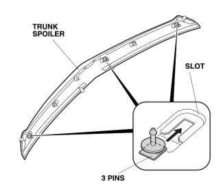
14. Install a thin seal (1 mm) to each of the three pins.
