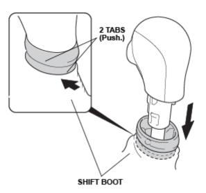
3. Pry out from the bottom of the shift knob cover and remove the cover.
