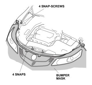
18. Attach the four hooks along the bottom of the mask to the bumper in the areas shown.
