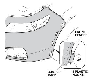
15. Attach the plastic hooks to the other fender the same way.
