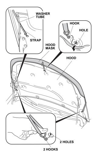
4. Attach the three hooks to the position shown.
