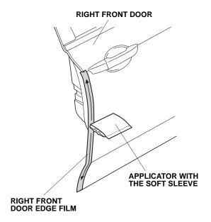
8. When you are satisfied that the door edge film is firmly attached to the edge of the door, slowly remove the outer protective film.
