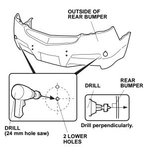
49. While wearing eye protection, drill the two inboard lower holes to 26 mm using a 26 mm hole saw. Drill from the outside of the rear bumper.
