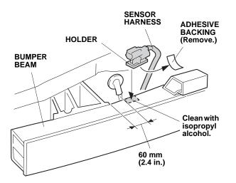
38. Remove the adhesive backing from the holder, and attach the holder at the position shown.
