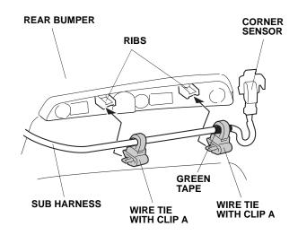
57. On the other side of the bumper, attach the wire tie with clip A to the sub harness at the green tape, and secure the sub harness to the ribs of the rear bumper using two wire ties with clip A.
