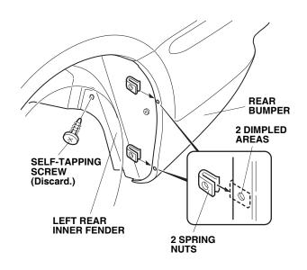
8. Position the left rear splash guard on the rear bumper and left rear inner fender, and tighten the three self-tapping screws in the order shown.
