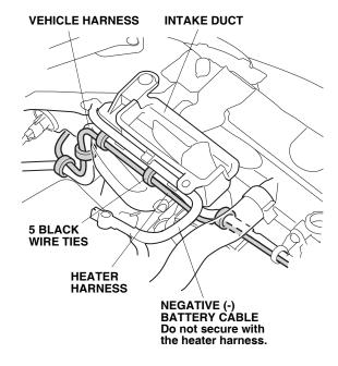
21. Using three black wire ties, secure the heater harness to the vehicle frame and vehicle harness.
