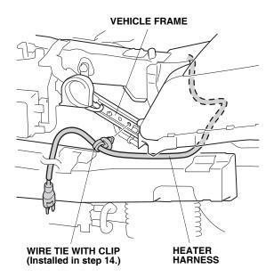
20. Secure the heater harness to the vehicle harness with five black wire ties.
