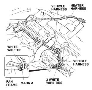
19. Using one wire tie with clip installed in step 14, secure the heater harness to the vehicle frame as shown.
