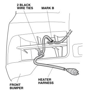
25. Attach the protective cap to the front bumper lower grille, and plug the heater harness connector into the protective cap.
