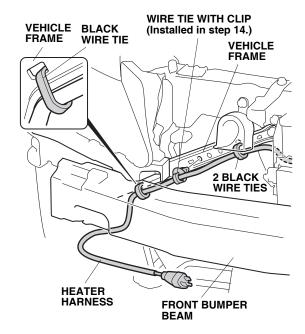
24. Using two black wire ties, secure the heater harness to the front bumper as shown.
