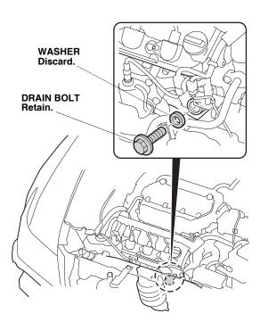
12. Install the aluminum washer and the engine block heater into the bolt hole using a 24 mm socket and a torque wrench. Torque the engine block heater to 60 N·m (44 lbf-ft).
