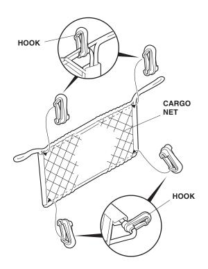
12. Install the cargo net to the tie down hooks and the anchors in the trunk. The cargo net can be installed in two different positions, vertically or horizontally.
