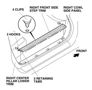
47. Pull away the right front door opening seal. Remove the right cowl side panel (two clips).
