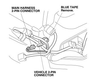
35. Using four wire ties, secure the main harness to the vehicle harness in the areas shown.
