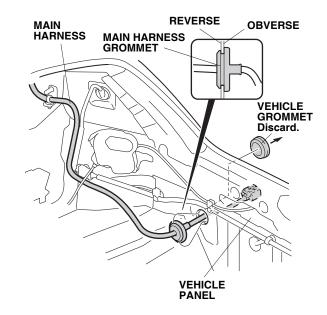
41. Using four wire ties, secure the main harness to the vehicle harness in the areas shown.
