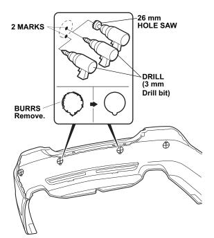
13. Install the one corner sensor (white) in the rear bumper using one sensor clip A.
