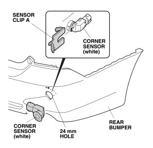
14. Install the one corner sensor (white) in the rear bumper using one sensor clip A.
