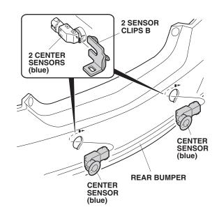
16. Plug the four subharness 2-pin connectors to the two corner sensors and two center sensors.
