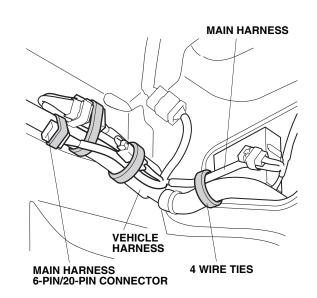
36. Insert the two main harness clips to the vehicle panel shown to secure the main harness.
