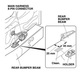
44. Plug the subharness 8-pin connector to the main harness 8-pin connector, then reinstall the rear bumper.
