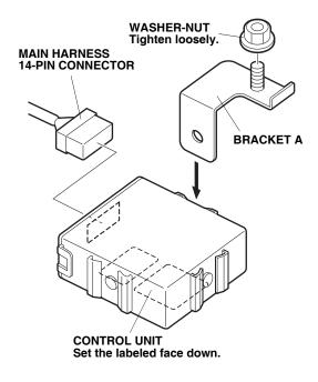
31. Install the control unit to the vehicle panel and tighten the washer-nut.
