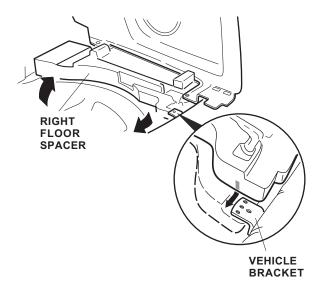
35. Loosely install one 6 x 20 mm flange bolt into the right jack nut.
