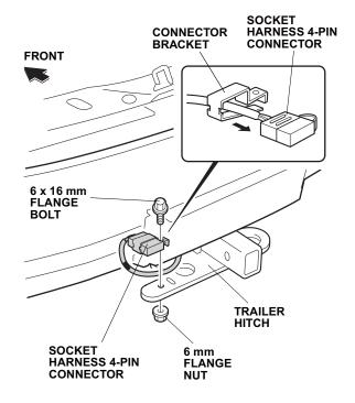
28. Secure the socket harness to the trailer hitch at the black tape using one wire tie.
