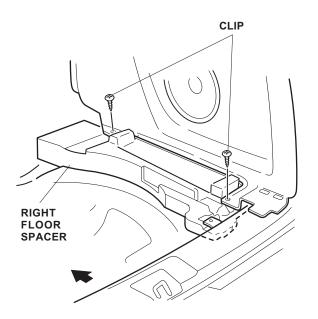
14. Remove the right floor spacer by gently pushing in at the back edge, and pulling out at the front edge to clear the vehicle bracket.
