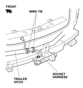
27. Attach the socket harness 4-pin connector to the trailer hitch using the 6 x16 mm flange bolt and the 6 mm flange nut.
