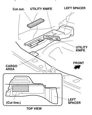
12. Locate the right spacer. Using an utility knife, cut out the right spacer as shown. Do not damage the vehicle harness under the right spacer.
