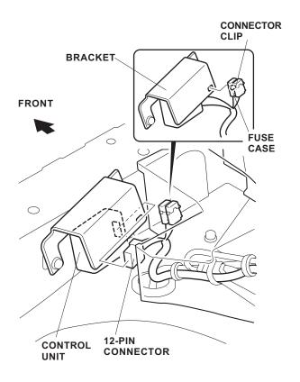
38. Rotate the control unit assembly down onto the right flange bolt. Torque both 6 x 20 mm flange bolts to 4.0 N·m (3.0 lb-ft).
