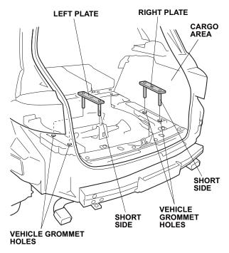
42. Install the two 12 x 40 mm bolts with plain washers and lock washers but do not tighten the bolts yet.
