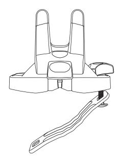
2. Position the base on the crossbar. Loosely install one bolt and knob as shown.
