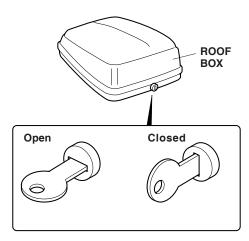
**Locking:** Press down on the lid. There should be an audible click. Be sure the lid is latched by attempting to lift the lid. Turn the key clockwise to lock the roof box. Remove the key while not in use. Be sure the straps do not dangle from the roof.
