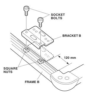
10. Attach one bracket A to each of four brackets (B), using two bolts, two washers, and two nuts for each bracket A. Do not tighten the bolts yet.
