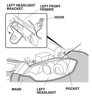
7. Secure one hook to the inside edge of the left headlight bracket.
