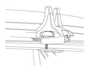
6. Slide the latch on one attachment strap into the clip on the base.
