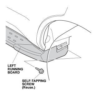
20. While pushing up on the left running board, secure the left front end cap with four of the self-tapping screws removed in step 2. Do not tighten the selftapping screws yet. (The right front end cap only uses three self-tapping screws.)
