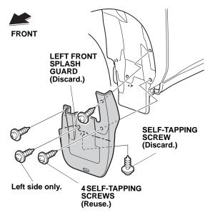
2. Remove the left front splash guard (five self-tapping screws).
