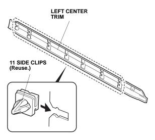
11. Hold the left center trim up, and fit the front clip and 11 side clips into the holes in the body, then push on the left center trim until the side clips snap into place.
