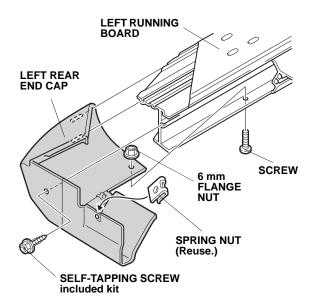
17. Install the spring nut to the left rear end cap.
