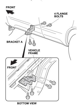
14. Position the two brackets B at the respective installation positions of the vehicle frame. Install the two brackets B on the vehicle frame with four flange bolts for each. Do not tighten the flange bolts yet. Make sure the flange bolts are installed in the correct positions.
