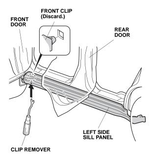
5. Using a clip remover, pry on the front clip from the back of the left side sill panel.
