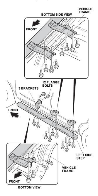
2. At the six flange bolts already attached to the left side step, torque the six flange bolts to 27 N·m (20 lbf·ft).
