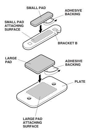
Using isopropyl alcohol on a shop towel, clean the four plates where the large pads will attach.
