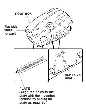
Attach an adhesive seal over each of the four unused mounting holes (two on each side) at the rear of the base of the box. The seals will help prevent water from entering the roof box. Remove the roof box. 4. Using isopropyl alcohol on a shop towel, clean four brackets B where the small pads will attach. Remove the adhesive backings from the small pads, and attach them to the brackets B.
