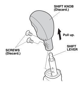
4. Install the new shift knob using the two new screws. Using a torque screwdriver, torque the screws to 3 N·m (18 lb-in). Do not overtighten the screws.
