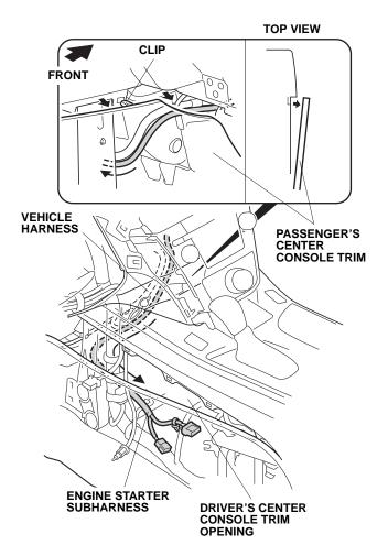
70. Secure the engine starter subharness to the vehicle harness with four wire ties in the areas shown.
