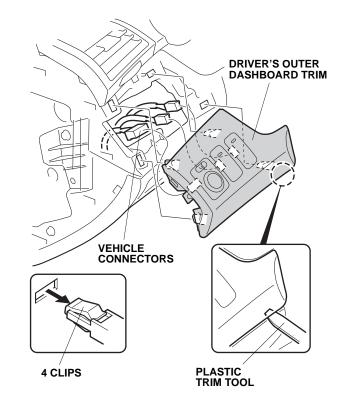
16. Using a plastic trim tool and a shop towel, remove the driver's center trim (five clips and three retaining tabs).
