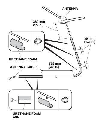
23. Using scissors, cut one urethane foam piece in half. Wrap the two halves of the urethane foam around the antenna cable at the measurements shown. 24. Measure and mark the antenna plate, using two pairs of needle nose pliers, bend the antenna plate to the angle shown.
