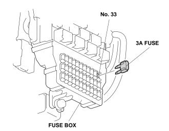
81. Using isopropyl alcohol on a shop towel, clean the area where the fuse label will attach. Attach the 3 A ENG STARTER fuse label to the No.33 slot on the inside of the fuse box lid.
