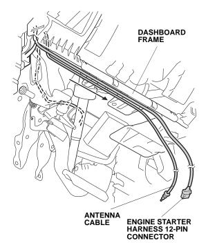
60. At the center console, route the engine starter harness 12-pin connector and antenna cable connector down along the vehicle harness to the driver's center console trim opening.
