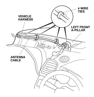
37. At the dashboard area, secure the antenna cable to the vehicle harness with one wire tie.
