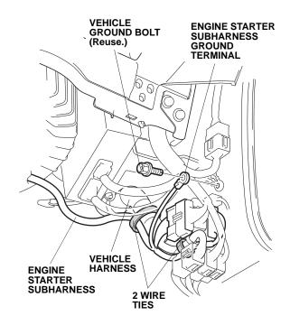
67. Secure the engine starter subharness to the vehicle harness with two wire ties.
