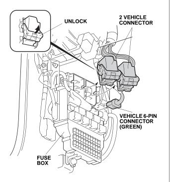
41. Unplug the vehicle 6-pin connector (green) from the fuse box.
