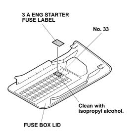
82. Using isopropyl alcohol on a shop towel, clean the area where the caution label will attach. Attach the caution label to the under side of the hood as shown.
