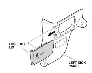
80. Install the 3A fuse included in the kit into the No. 33 slot of the fuse box.
