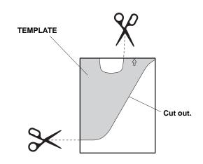
26. Secure the template to the windshield with the masking tape by aligning it with the edge of the black ceramic part as shown.
