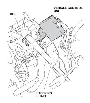
48. Route the two engine starter harness 14-pin connectors over the steering shaft.
