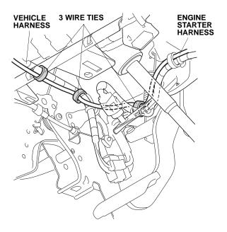
57. Secure the engine starter harness 6-pin connector (green) to the vehicle harness with one wire tie. Near
