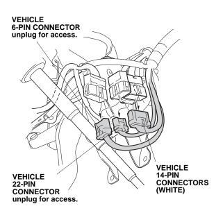
50. Plug the engine starter harness 14-pin connector into the vehicle 14-pin connector and plug the
