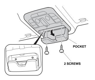
6. Using a plastic trim tool, remove the roof console (two clips and unplug three vehicle connectors).
