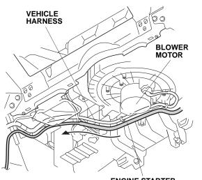
ENGINE STARTER SUBHARNESS 69. Pull the end of the passenger's center console trim to release the one clip shown. Route the engine starter subharness along the vehicle harness to the driver's center console trim opening.
