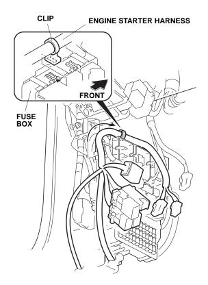
43. Plug the engine starter harness 6-pin connector (green) into the fuse box, and plug the vehicle 6-pin connector (green) into the engine starter harness 6-pin connector (green).
