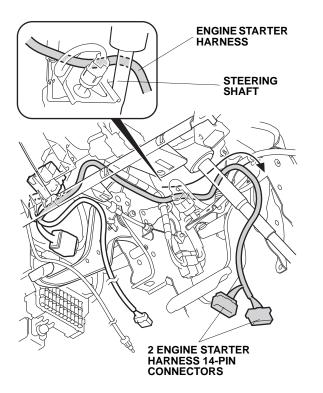
49. Directly behind the steering shaft, unplug the vehicle 22-pin connector and 6-pin connector for access, and the vehicle 14-pin connector (white).
